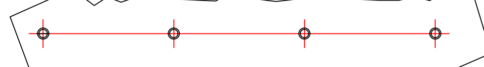
VIEW OF LV SIDE - CABLE CLEAT STUDS CABLES MUST BE SUPPORTED IN ACCORDANCE WITH - CURRENT IET Wiring Regulations BS7671 & IEC 61914
