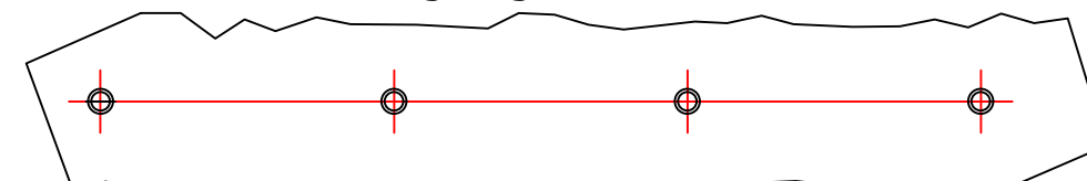
VIEW OF LV SIDE - CABLE CLEAT STUDS CABLES MUST BE SUPPORTED IN ACCORDANCE WITH - CURRENT IET Wiring Regulations BS7671 & IEC 61914
